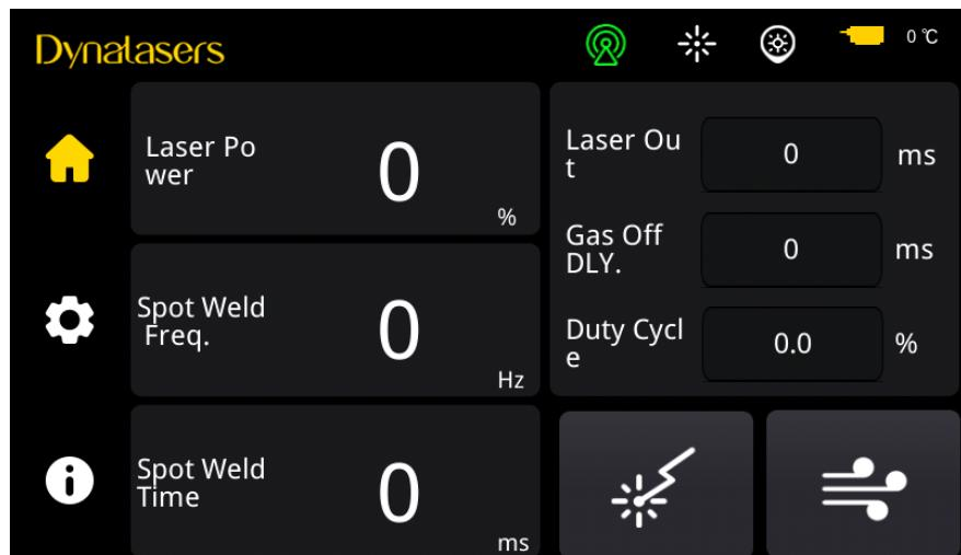
•Home Page: Configure laser power, pulse frequency, pulse duration, laser delay, and gas shut-off delay.
