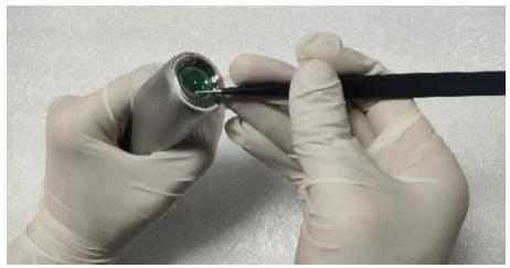
7. Replace the cleaned lens into the gun body;
