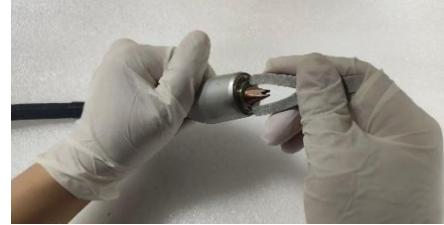
12. Use the Y-shaped tool to tighten the locking ring;
