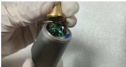
9. Align the air vent beneath the copper nozzle
