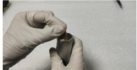
10. Press the nozzle into the gun body;
