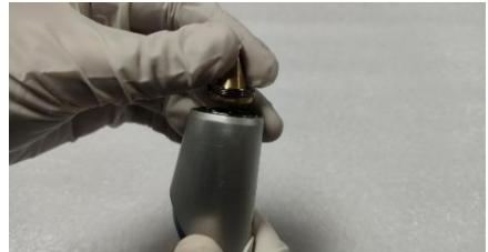
1. Use the Y-shaped tool to loosen the locking ring clockwise and remove it;
